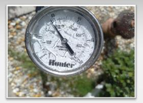
Pressure testing will be done at each control valve and at the head locations furthest away from the valve.
